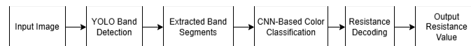
Fig. 10. Proposed YOLO-CNN hybrid architecture for future localized resistor band detection and color classification
