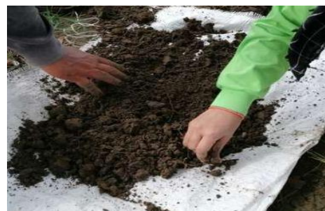
Fig. 6. Arranging the soil aggregate to assess soil structure
