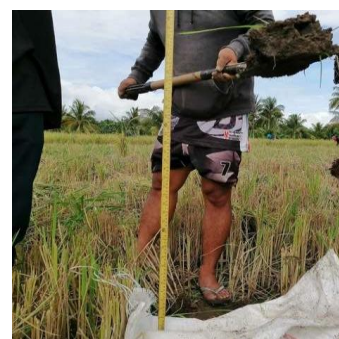
Fig. 5. Dropping the soil sample for the shatter
